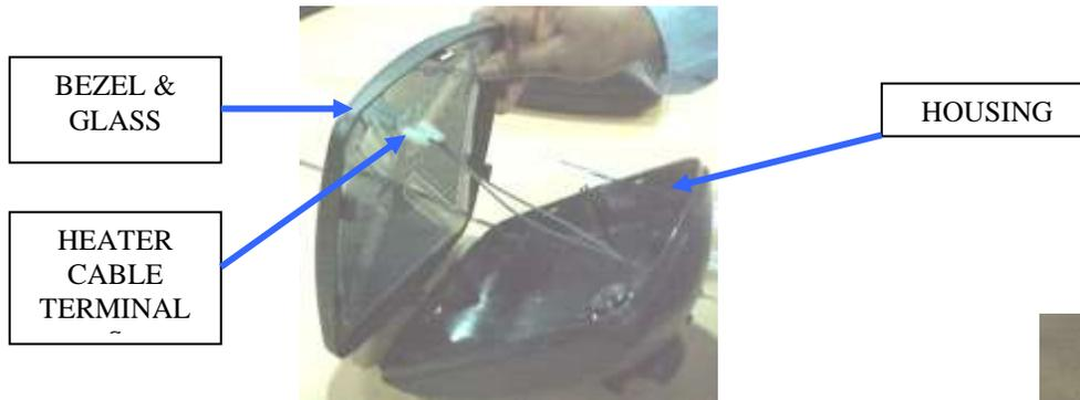
Remove Head heater cable from housing (remove 2 screws).
