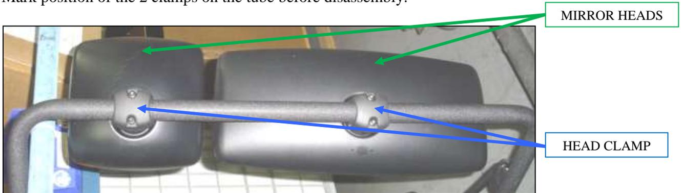
Remove the head clamp screws and the clamp(s). Make sure to save them for re-assembly.
