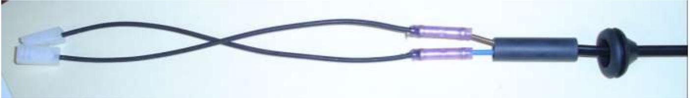
Cover the splice seals with the heat shrink tubing.
