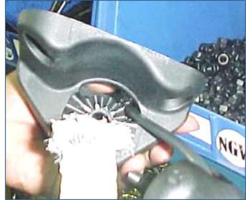
Slide the bolt through the tube connector.
